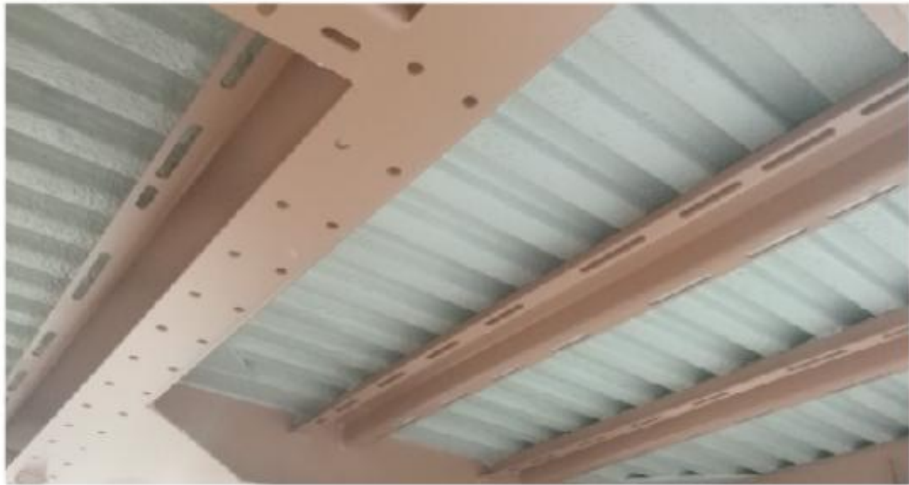
Air++3101D is applied to the underframe of the train
