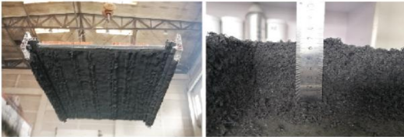
Expansion effect after fire prevention experiment (Complete carbonization layer)
